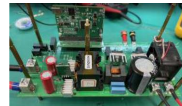
Benchmark For Server 1KW Solution
